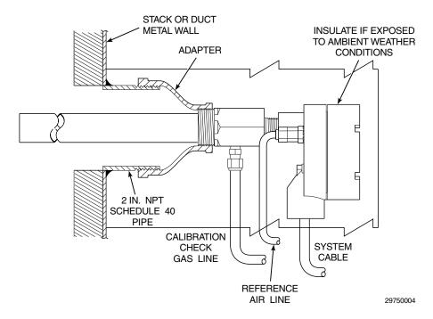
Figure 2-4. Horizontal Probe Installation
